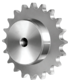
3/4"x7/16"- 12B-1 rullo 12,07 mm - Dimensioni - Dimensions - B1=11.1 / C=2 / r3=19
